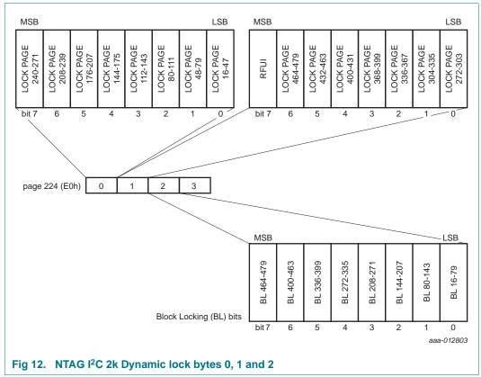
The default value of the dynamic lock bytes is 00 00 00h. The value of Byte 3 is always 00h when read.
