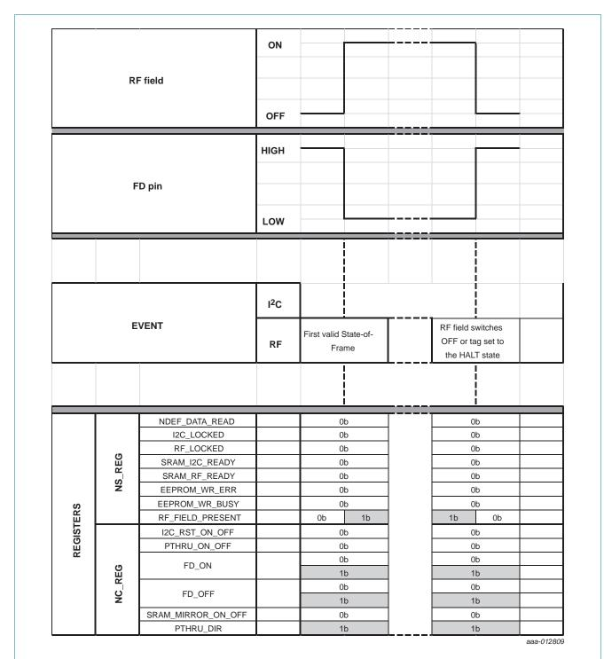
Fig 16. Illustration of the field detection feature when configured for First valid state of Frame detection
