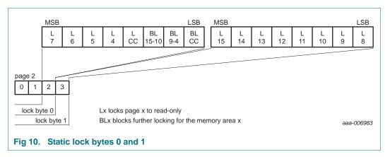
For example, if BL15-10 is set to logic 1, then bits L15 to L10 (lock byte 1, bit[7:2]) can no longer be changed. The static locking and block-locking bits are set by the bytes 2 and 3 of the WRITE command to page 02h. The contents of the lock bytes are bit-wise OR'ed and the result then becomes the new content of the lock bytes.
