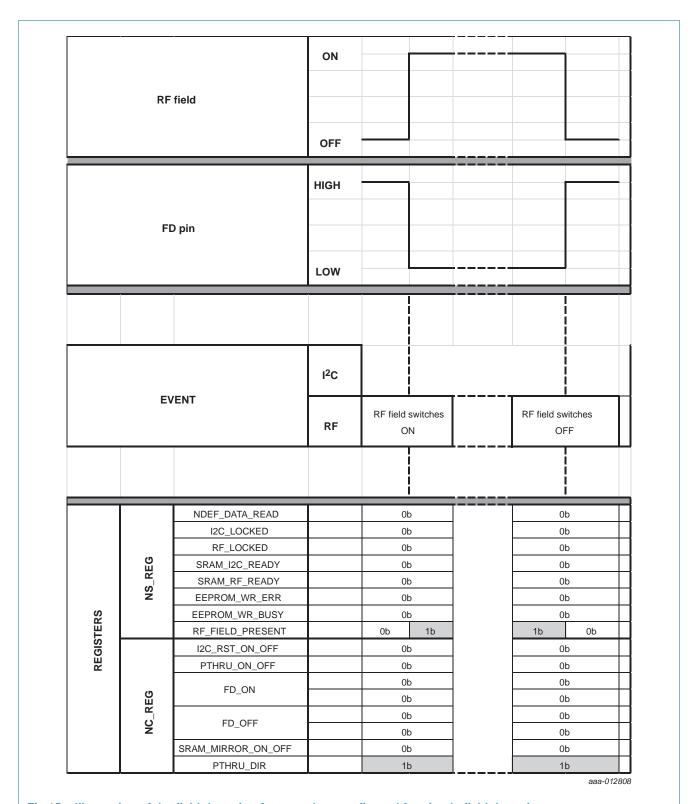
Fig 15. Illustration of the field detection feature when configured for simple field detection
