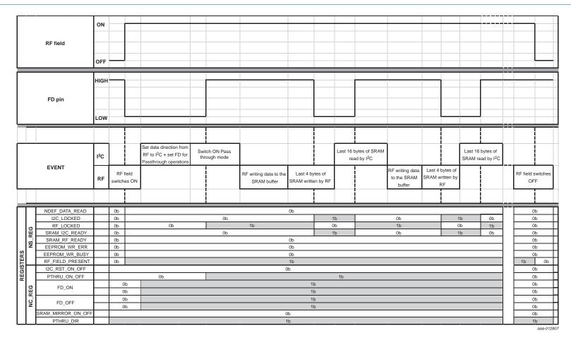
Fig 31. Illustration of the Field detection feature in combination with the Pass Through mode for data transfer from RF to I2C
